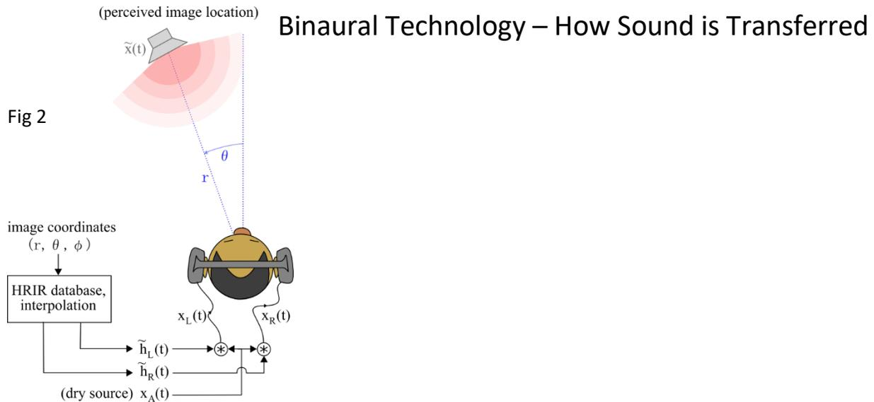
Binaural technology takes HRIR database and interpolates in where the sound it should be mimicked. Fastcomcorp took the same approach as binaural technology has done through the image coordinates and HRIR database. FDA's interpolation process is more advance and complex. Before we go further one must understand the Cartesian coordinate system, points (X,Y,Z). Because it will help one adapt the following information.
