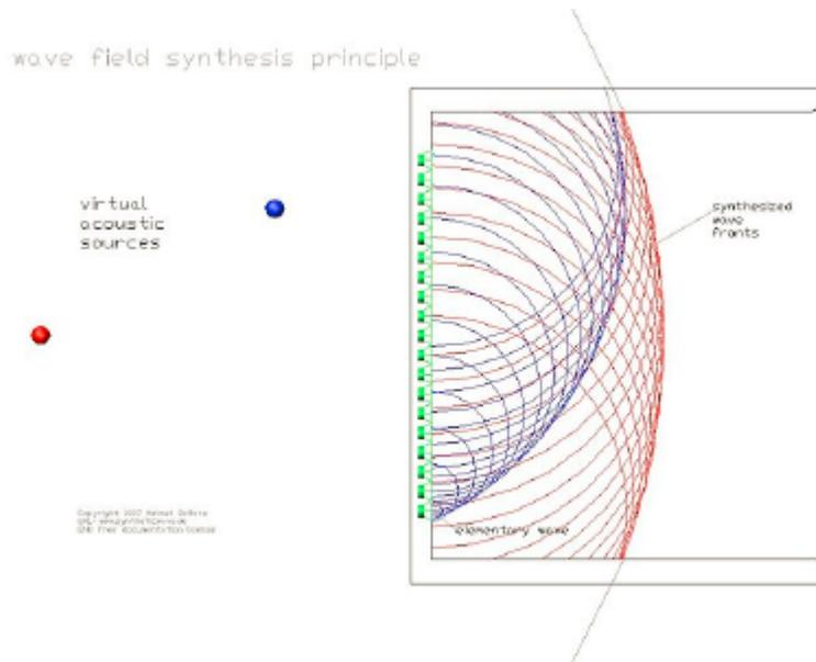
It is based on **Huygens' Principle** which states that any wave front can be regarded as a superposition of elementary spherical waves. Which can be synthesized from such elementary waves, this is backed by **The Kirchhoff-Helmholtz Integral**. WFS is a spatial audio rendering technique, characterized by creation of virtual acoustic environments.
